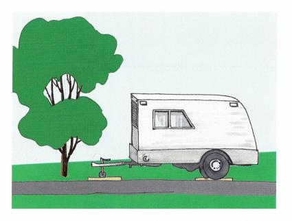
Excessive weight from large heavy vehicles can depress your new driveway. Keep oil trucks, concrete trucks and any other heavy trucks off your new driveway. When storing campers and boats for long periods of time, place a piece of plywood under the tongue jack and also under the tires.
