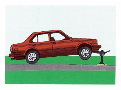
Avoid using jack stands or car ramps unless a piece of plywood is placed under them to help distribute the weight.
