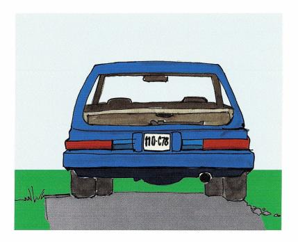
The edges are the weakest part of your driveway due to the lack of side support. Avoid driving on the edges since they will crack and crumble in time. We suggest building up the sides of your driveway with topsoil to approximately one inch from the top of the driveway to allow room for sod growth and water drainage. This will support the edges and enhance the appearance after grass is grown.
