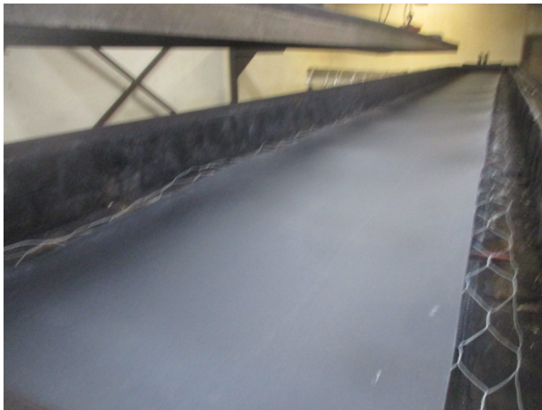
Photo No. 2 Unexposed Surface of the Test Specimen (Pre-test)
