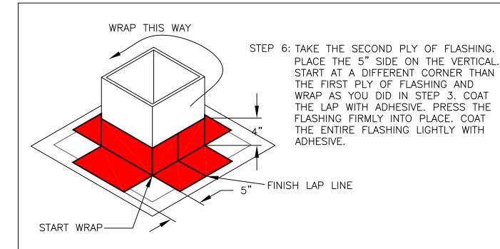
NOTE: LAURENCO PMMA LIQUID FLASHING MAY BE UTILIZED IN LIEU OF MEMBRANE FLASHING.
