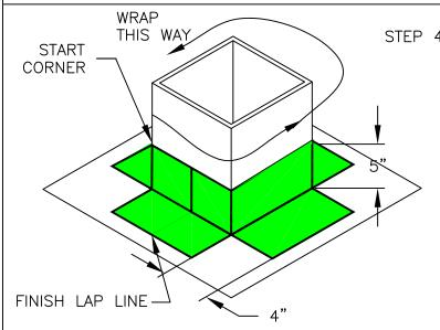
STEP 4: TAKE THE FIRST PLY OF FLASHING. MAKE SURE THE 4" SIDE IS ON THE VERTICAL. STARTING FLUSH AT A CORNER WRAP THE SHEET AROUND THE PENETRATION. MAKE SURE THE WRAP GOES COMPLETELY AROUND AND OVER LAPS ITSELF. PRESS THE FLASHING FIRMLY INTO PLACE. COAT THE LAP AREA LIGHTLY WITH ADHESIVE. COAT THE ENTIRE FIRST PLY LIGHTLY WITH ADHESIVE.
