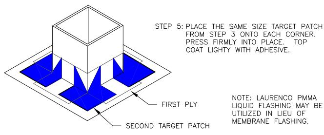
FROM STEP 3 ONTO EACH CORNER. PRESS FIRMLY INTO PLACE. TOP COAT LIGHTY WITH ADHESIVE.
