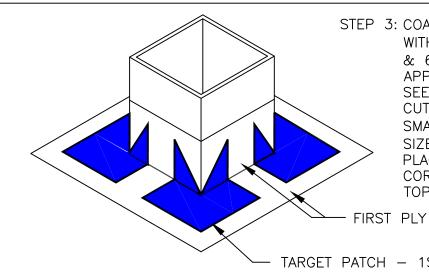
STEP 3: COAT THE RECTANGULAR PENETRATION WITH ADHESIVE 6" UP THE VERTICAL & 6" OUT ONTO THE HORIZONTAL IF APPLICABLE. SEE DETAIL 24 STEP 13 FOR CUTTING THE TARGET PATCH. FOR
