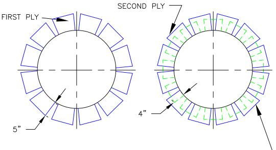
PIG-EAR FLASHING FLANGE ONTO WALL OR DECK-STAGGER PIG-EARS FOR FULL COVERAGE
