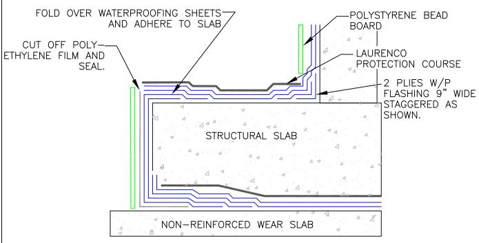
STEP#2 - PLACE SLAB THEN FOLD OVER WATERPROOFING SHEETS AND ADHERE TO THE TOP OF THE SLAB.
