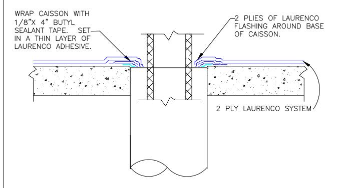
NOTE: USE OF THIS DETAIL REQUIRES PRIOR APPROVAL FROM LAURENCO TECHNICAL DEPARTMENT. DETAIL IS ONLY TO BE USED WHEN THE STRUCTURAL ENGINEER WILL NOT ALLOW FULL WATERPROOFING MEMBRANE SYSTEM ACROSS THE TOP OF THE CASSION.
