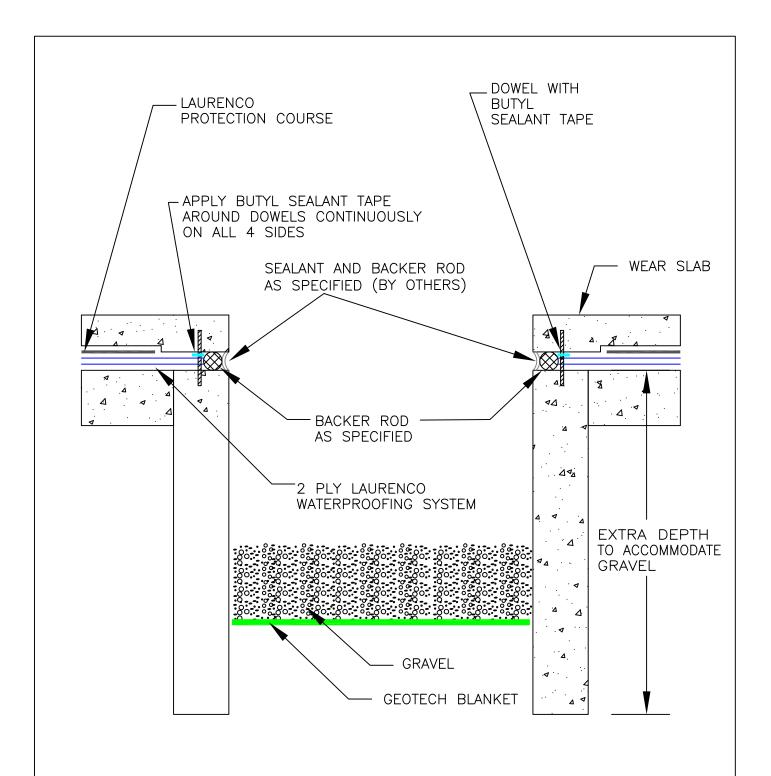
NOTE: USE OF THIS DRAWING DEPENDS ON THE DEPTH OF THE WATER TABLE. SEE SUMP AND ELEVATOR PIT DETAIL 224 WHERE THERE IS HEAD PRESSURE WITH NO DRAINAGE.
