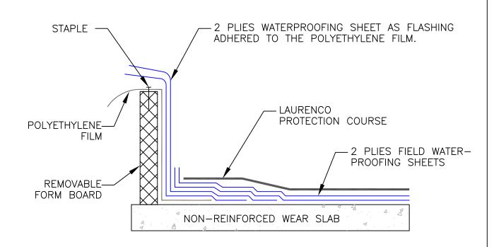
STEP #1 - APPLY POLYETHYLENE FILM, WATERPROOFING AND PROTECTION COURSE AS SHOWN.
