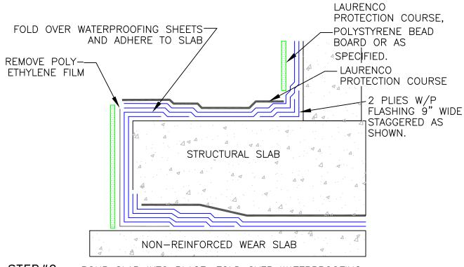
STEP#2 — POUR SLAB INTO PLACE. FOLD OVER WATERPROOFING SHEETS AND ADHERE TO THE TOP OF THE SLAB.
