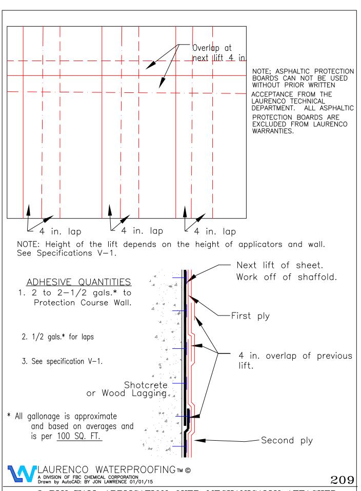
2 PLY WALL APPLICATION OVER MECHANICALLY ATTACHED ASPHALTIC PROTECTION BOARD
