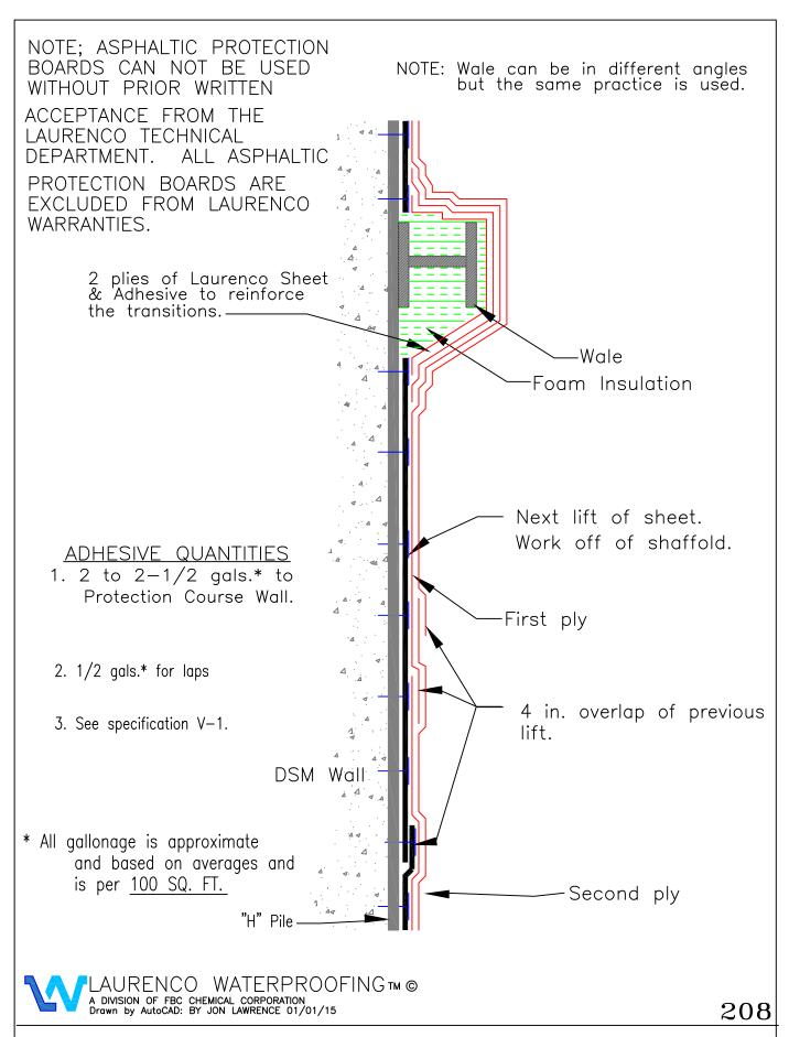
2 PLY WALL APPLICATION OVER MECHANICALLY ATTACHED ASPHALTIC PROTECTION BOARD
