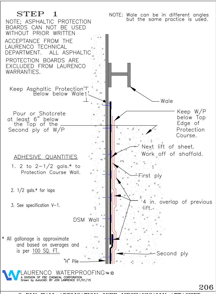
2 PLY WALL APPLICATION OVER MECHANICALLY ATTACHED
