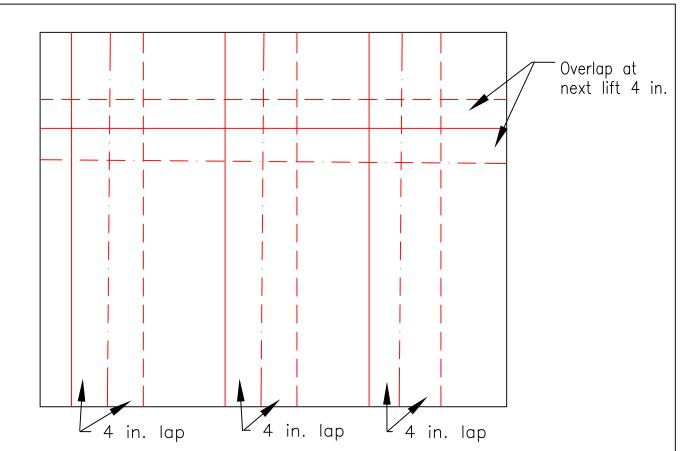
NOTE: Height of the lift depends on the height of applicators and wall. See Specifications  $V\!-\!1.$
