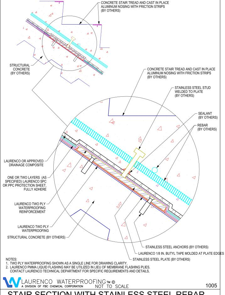
STAIR SECTION WITH STAINLESS STEEL REBAR CAGE MOUNTING BRACKET ASSEMBLY FLASHING
